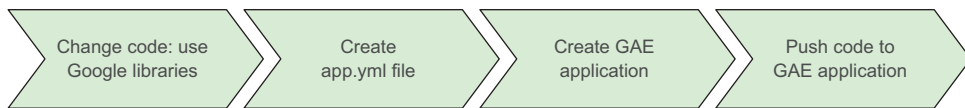
Figure 10.2 Steps to deploy on the Google App Engine. First change the code to use Google libraries and create the app.yml configuration file. Then create the application and push it to the GAE.
